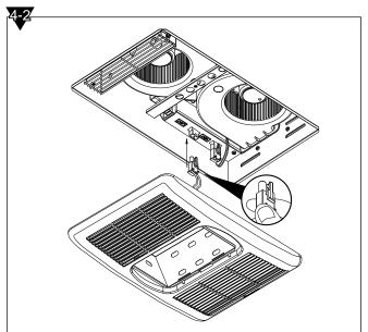
c. Install the Grille Assembly 2 into the Fan Body 1 using the Machine Screw 3.
